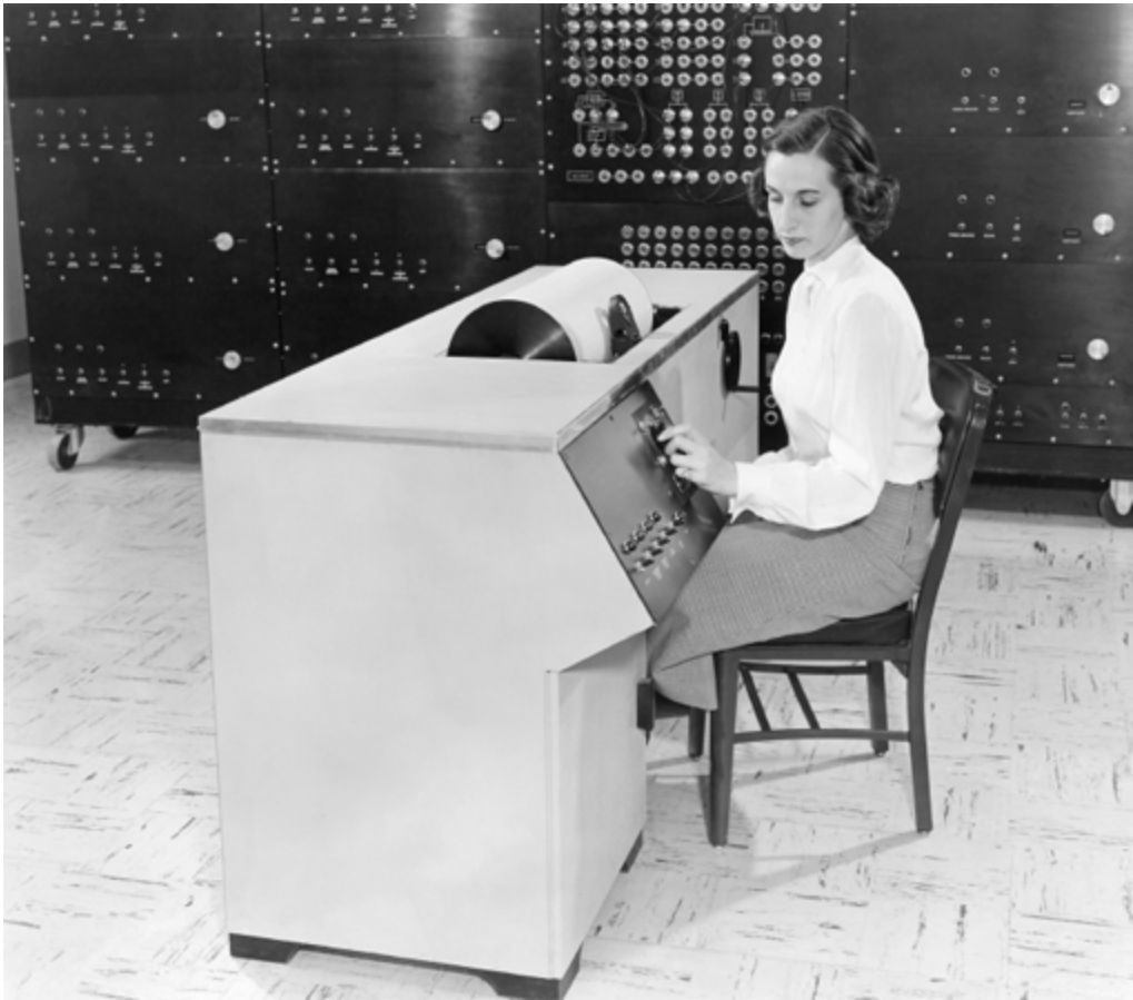
A differential analyzer at the Lewis Flight Propulsion Laboratory, in 1951. The analyzer was among the first advanced computing devices to be used for practical applications such as the design of bombs used to destroy German dams during World War II.
