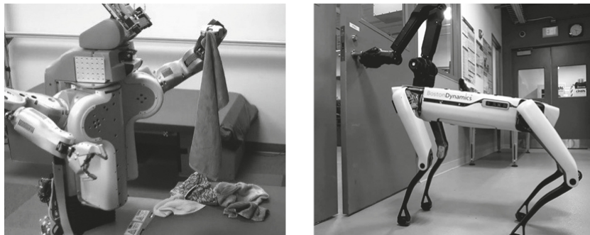
FIGURE 5: (left) BRETT folding towels; (right) the Boston Dynamics SpotMini robot opening a door.
